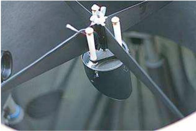
The secondary mirror is 3.1" which translates into a 20% central obstruction, and overall I find it quite acceptable for all types of viewing – lunar and planetary as well as DSO's. Some folks will talk about a contrast loss because the secondary isn't as small as it could be. In comparison with my other scopes, the 18" will (in good seeing) simply blow them out of the water in all respects – aperture rules. When compared to similar size
