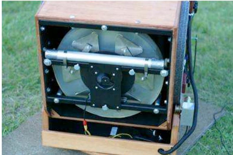
Obsession uses a low profile design with the truss poles mounted on the outside of the mirror box to shrink the overall size and weight of the box. Everything is low profile –
